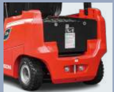
Battery is placed at the rear of the truck
