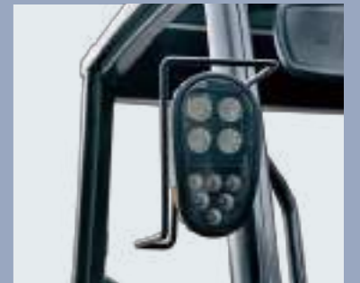
The new efficiency lighting system employs LED illuminant and new type reflector to reduce energy consumption, improve significantly illumination performance and prolong work time
